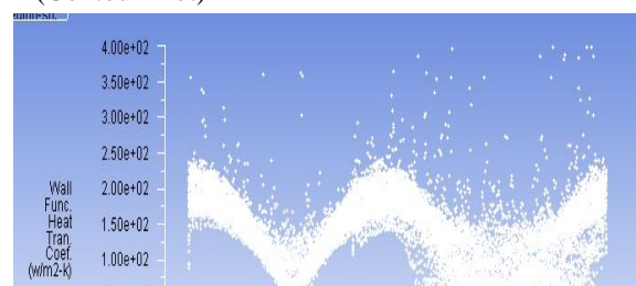
Fig. 10 Circular Fin – Heat transfer coefficient (Scatter Plot)
